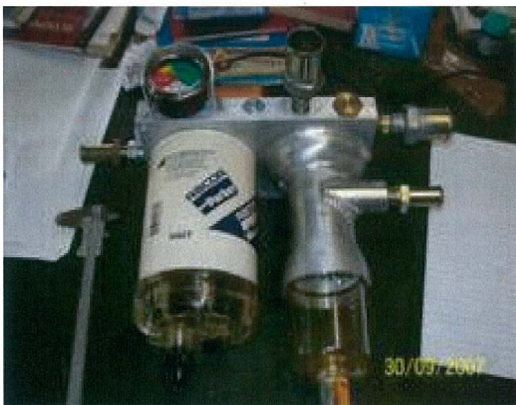
The heat exchanger and filter system
