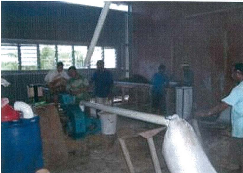
Re-shredding the copra waste to produce a powdered stock feed mix
